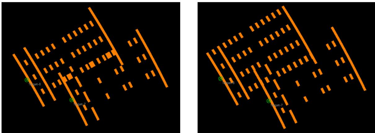
**Figure 2: Non-synchronous garbling (left) of two transponder replies. The response pulses do not align with allowable positions and may therefore be resolved. Contrast with synchronous garbling (right) where the overlapping pulses are in valid positions.**
