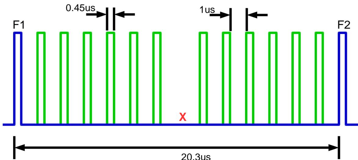
Figure 1: IFF response pulse positions, showing the framing pulses (F1 and F2) and the fixed possible positions of up to twelve pulses in between, which represent the encoded reply information.
